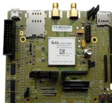
Fig. 3. Shield Modem 4G LTE[18]
